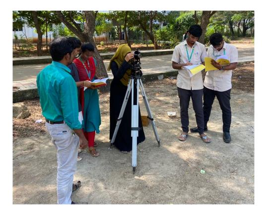
Theodolite is an instrument for measuring both horizontal and vertical angles, as used in triangulation networks. This activity in our course delivers the knowledge about the measurement of horizontal included angle between several points and vertical angle of various points. By measuring these angles, we can easily calculate the area of a particular plot and can find out the height of immeasurable things like electrical towers, tall buildings, small hills etc,
